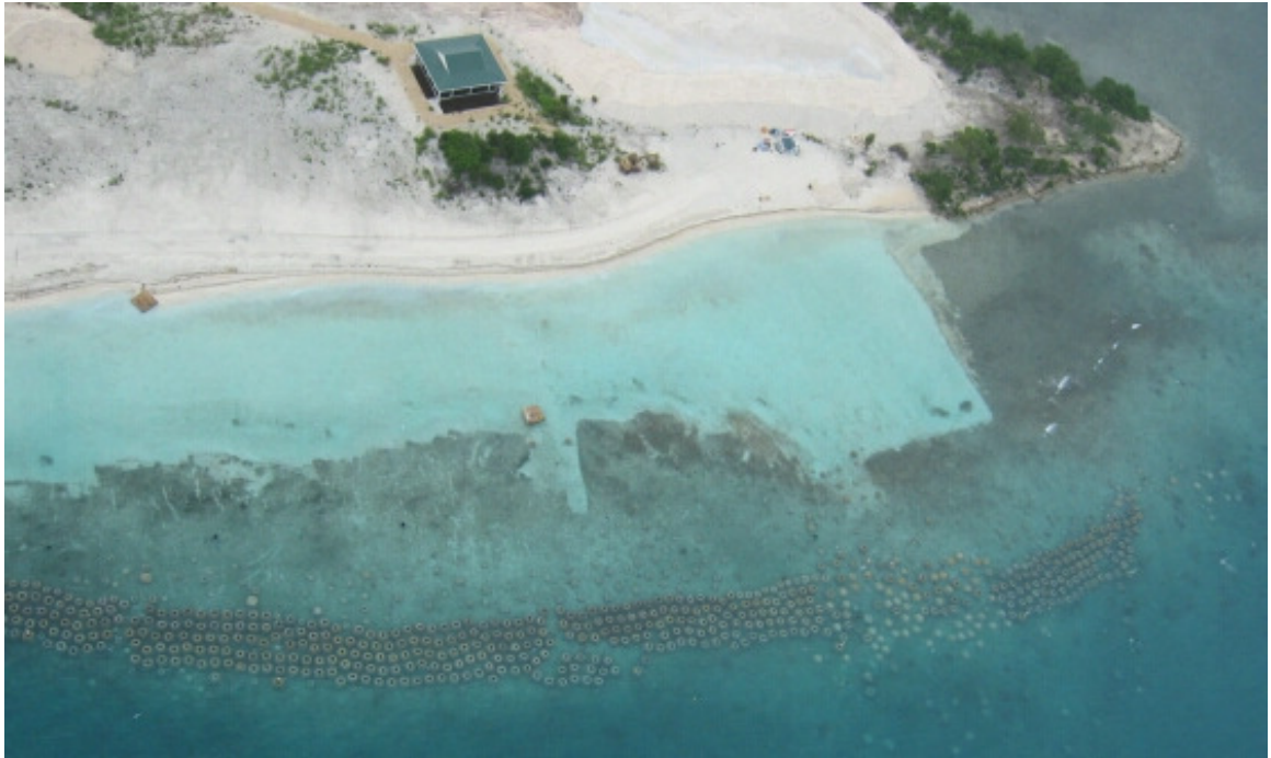
Figure 14. Aerial Photograph of 5-Row Reef Ball Breakwater in Antigua The breakwater also incorporates snorkel trails, swimming and diving areas.)
