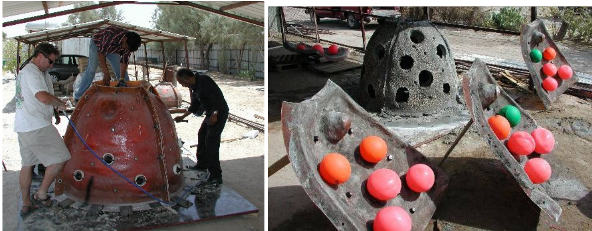
Figure 2. Traditional Reef Ball Unit Mold Fabrication
